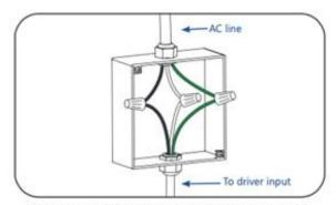
Connect the green wire to the incoming ground conductor. Connect the black wire to Line 1 and white wires to Neutral or Line 2 of the incoming AC line.
